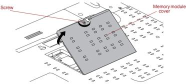
Figure 3-6 Removing the memory module cover
